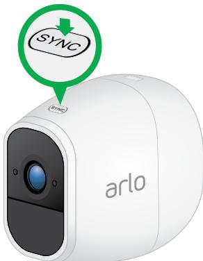
The LED on the camera blinks slowly when the sync process starts. The blue LED blinks rapidly to confirm syncing.
