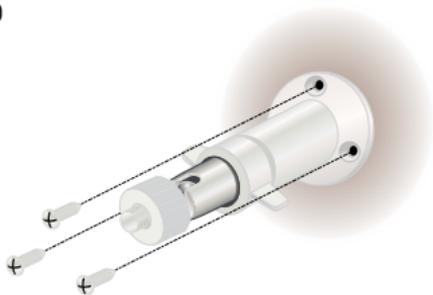
2. Tighten the metal collar on the mount to secure the post.
